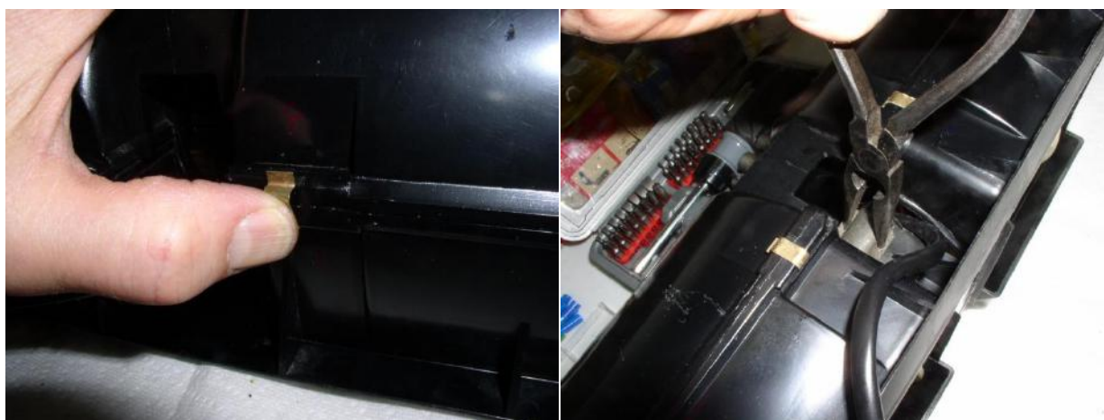
Figure 17. Install eight small and two large housing clips. The large clips should be spread by a pair of snap ring pliers to make installing them easier and avoid stressing the plastic housing.
