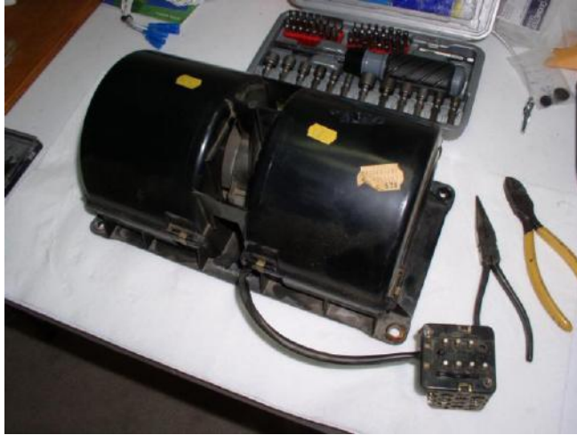
Figure 4. Untouched for the twenty-three years after it left the factory, my '87 560 SL's heater blower unit was long overdue for a refresh. Noisy and arthritic in operation, one motor bearing was stiff and the other worn out with about \frac{1}{4} " (6mm) of radial play at the fan.
