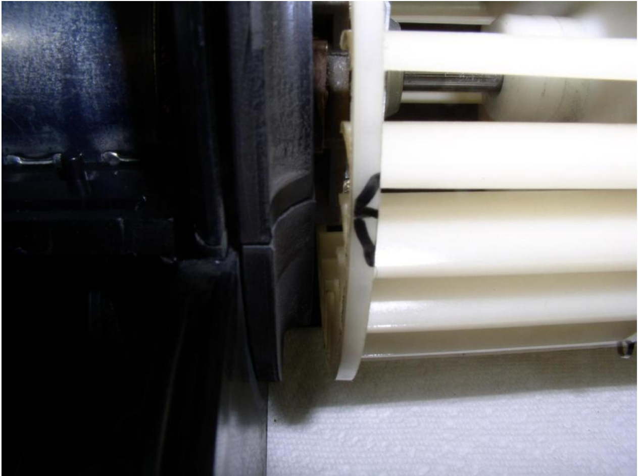
Figure 15. It's IMPORTANT to ensure each fan edge has at least about 1/8" (3mm) clearance from its guide. Despite careful measuring and marking, I had to readjust one of my fans slightly outward on its shaft to better clear its inside guide.
