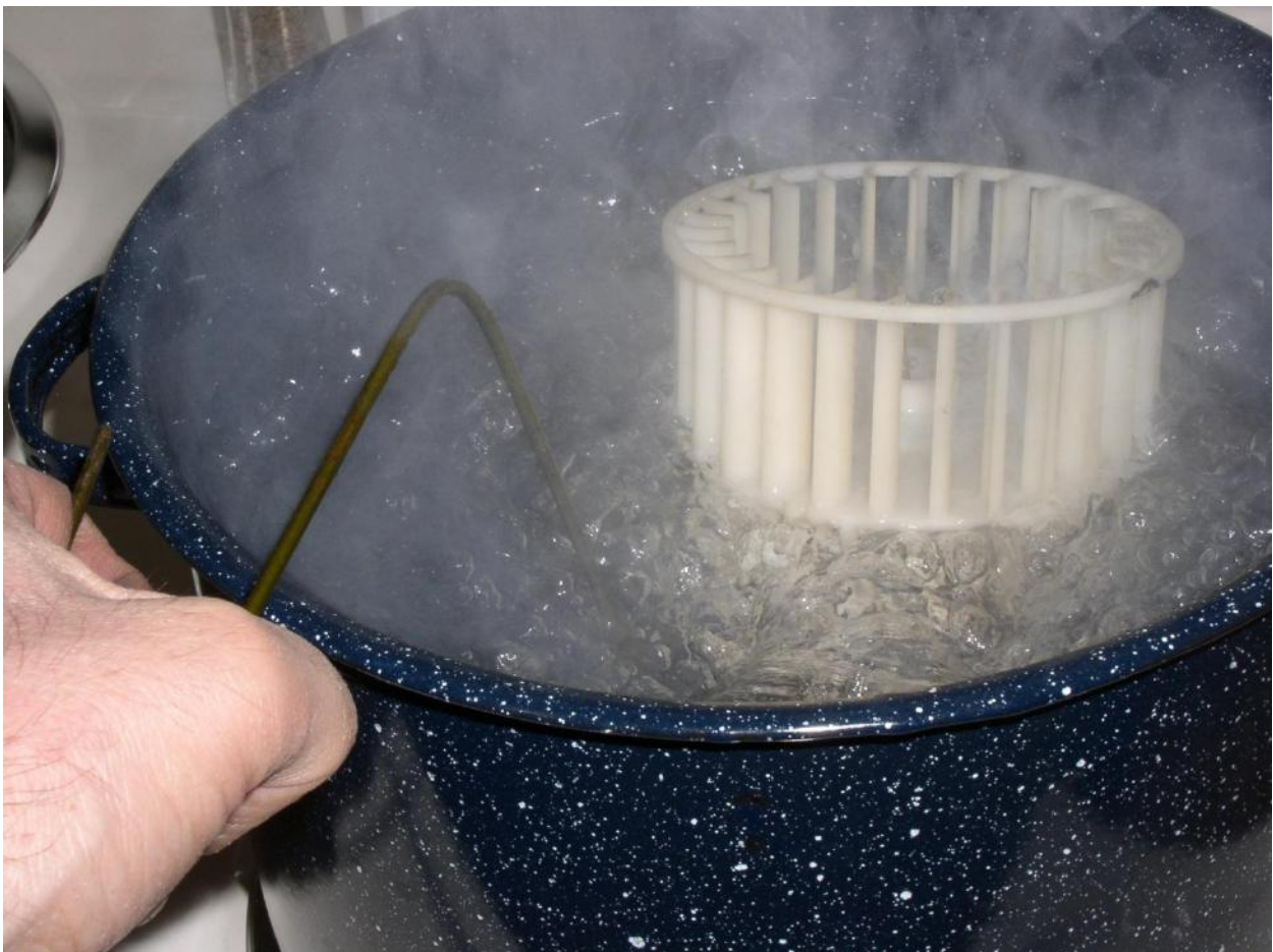
Figure 11. Boiling the fans before pressing them on their shafts makes installation easy...and precludes the expensive breakage that can quadruple the cost of this repair!
