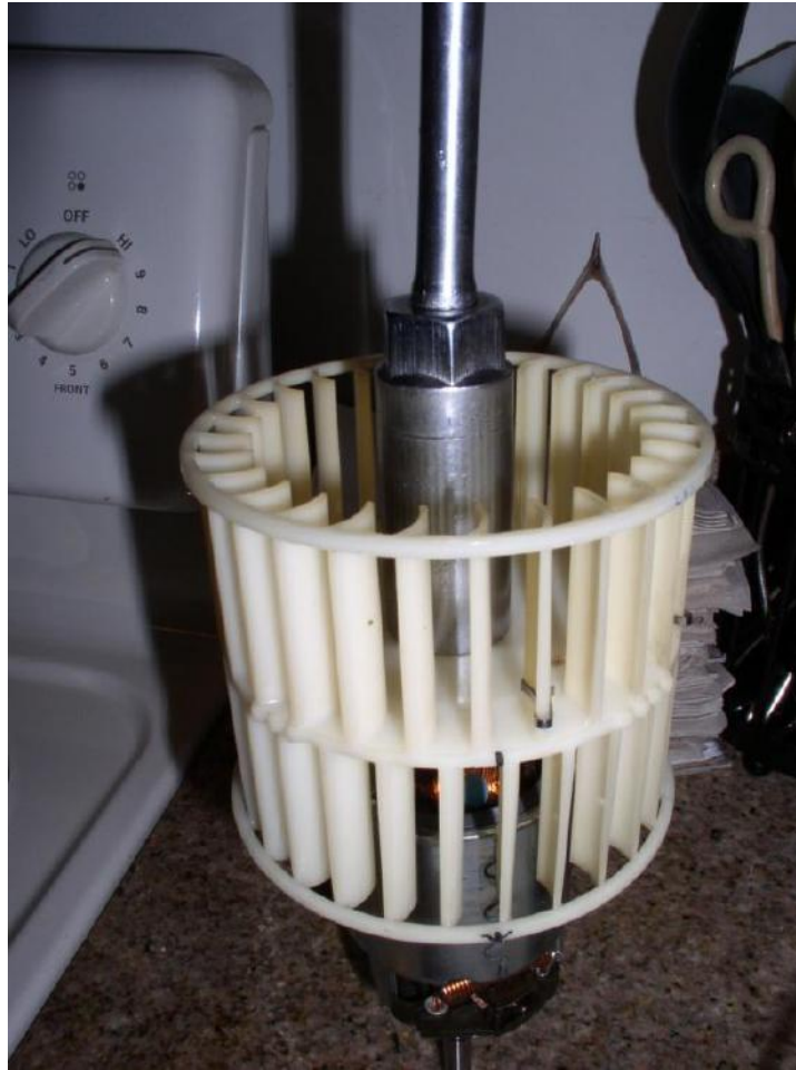
Figure 12. An improvised mandrel presses the left fan onto its shaft without putting pressure on the motor's bearings.
