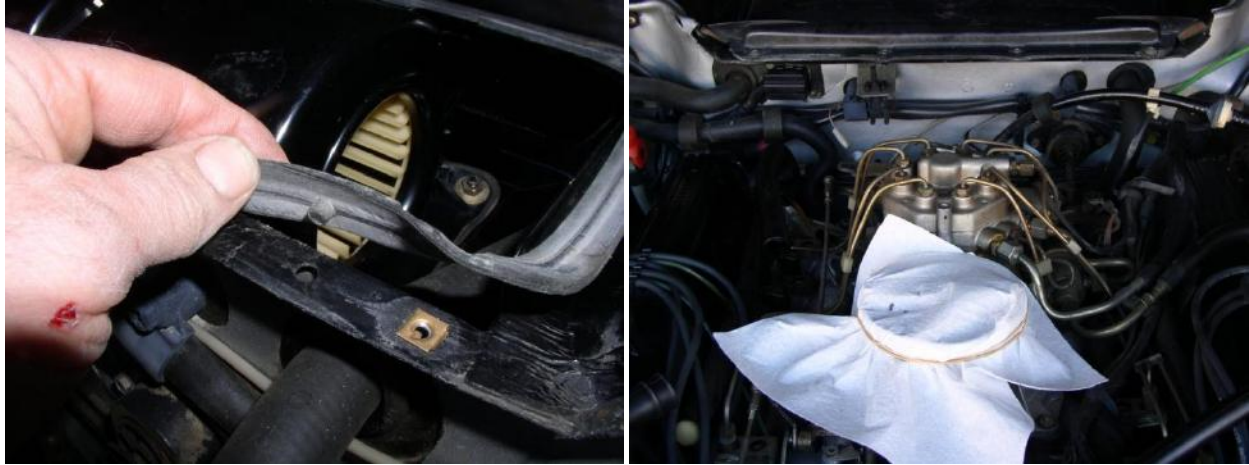
Figure 19. The top cover gasket must be installed only one way for these nubs to line up with their holes. When the cover is screwed down, remove the engine air intake covering and reinstall the air cleaner.
