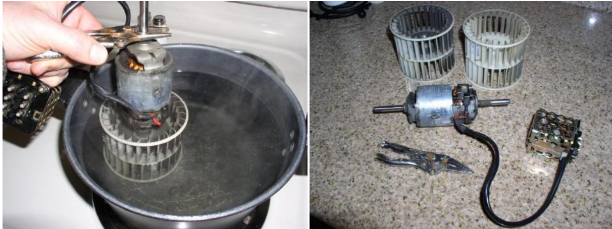
Figure 9. Boiling water expands the plastic fans at a safe, controlled temperature, 212 F (100C), allowing them to be removed from the motor shaft without the excessive, ill-applied force that often breaks them--and your wallet!
