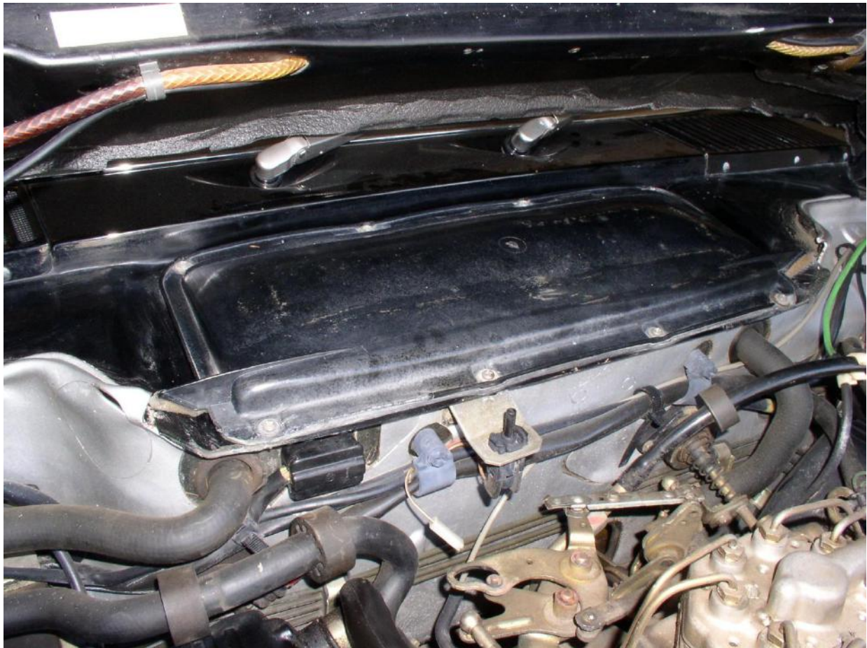
Figure 1. After removing the air cleaner and sealing the engine air intake, remove the eight Phillips screws that hold the heater blower motor well cover plate in place. Remove the cover and gasket. Unplug the blower motor cable.
