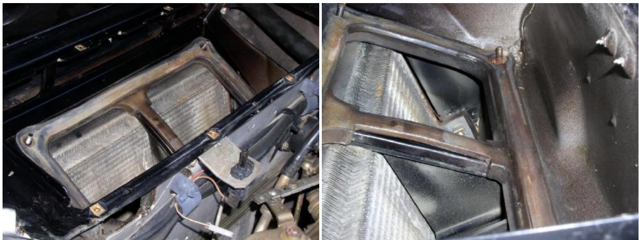
Figure 3. Four M6 studs hold the heater blower housing in the well. After blower unit is removed, inspect the condition of the rubber gasket. Look for and remedy any rust issues you discover, and give the well a good cleaning.
