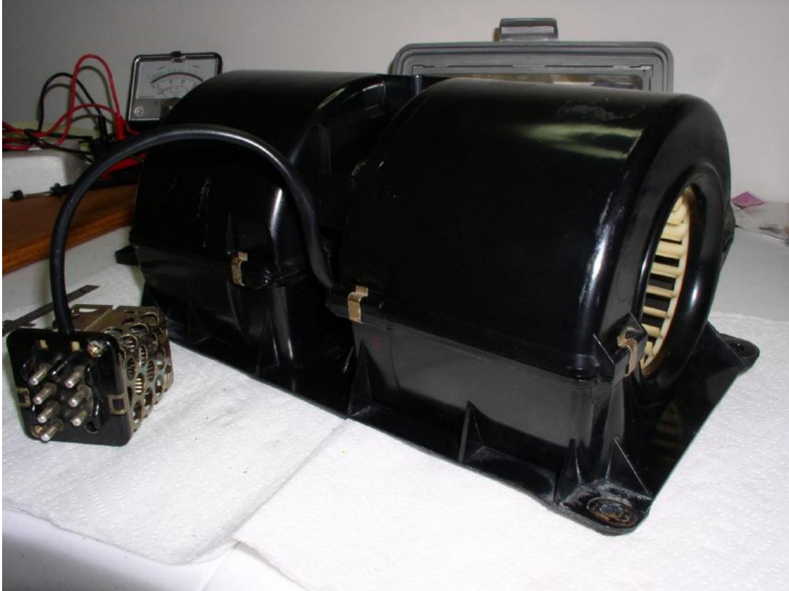
Figure 18. With a fresh new Bosch motor, the blower unit is ready for installation.
