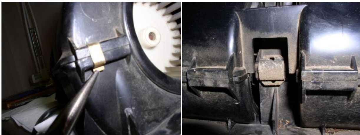
Figure 5. Remove the eight small and two large clips that hold the clamshell halves of the unit together.
