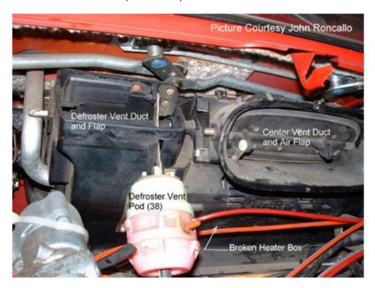
Here is what greeted owner, John Roncallo, when he removed the console and dash. Note the deteriorated defroster flap foam seal and the cracked heater box.
