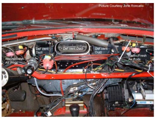
attach. Notice the def pod. See how the vacuum line tees at the center, and runs to the center pod. This shared vacuum line is why diagnosis is somewhat difficult. A leak in either renders both inoperative.
