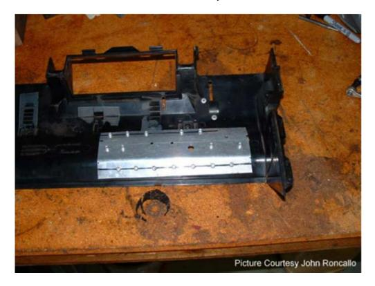
Here the owner has removed the heater box (actually the front half of the top half) and turned it inside up. He then applied a thin sheet metal backing with blind rivets, to repair the cracked housing.
