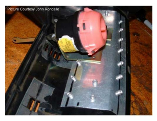
Here is the repaired housing with the center pod mounted in place. This is a view of the Inside of the top 1/2 of the heater housing.
