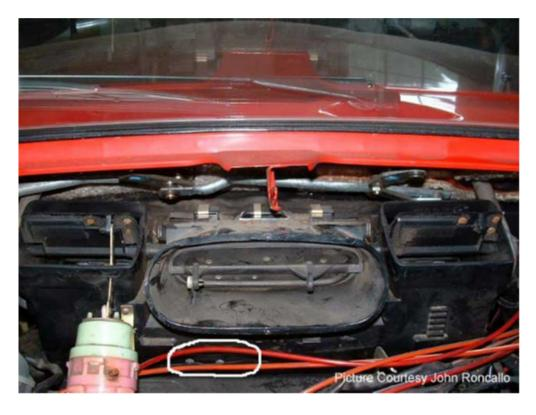
Another view of the top half of the heater box, prior to any repairs. The circled area is where the center pod mounts, and is visible when the radio is removed. Notice how a section of the heater box is completely nroken loose, and dislodged downward as to hide about 1/2 of the mounting rivets.
