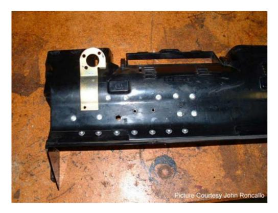
Here is the repaired housing from the front view. Note the size of the cracked portion of the housing, just visible around the two rivet holes. The larger hole to the left and a bit lower is where the vacuum line attaches to the pod after it is mounted inside.
