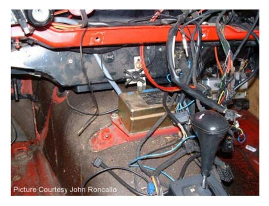
Here is the lower half of the heater box prior to any repairs. You can just see the cracked heater box at the top of the picture.
